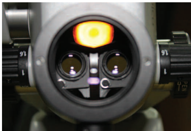
Figure 9 - Objective lens with the light on. The light comes out from the objective lens and takes a path parallel to the visual path.
