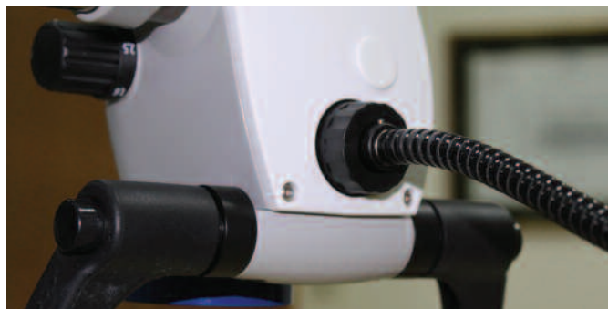
Figure 10 - Fiberoptic cable entering on the microscope body.
